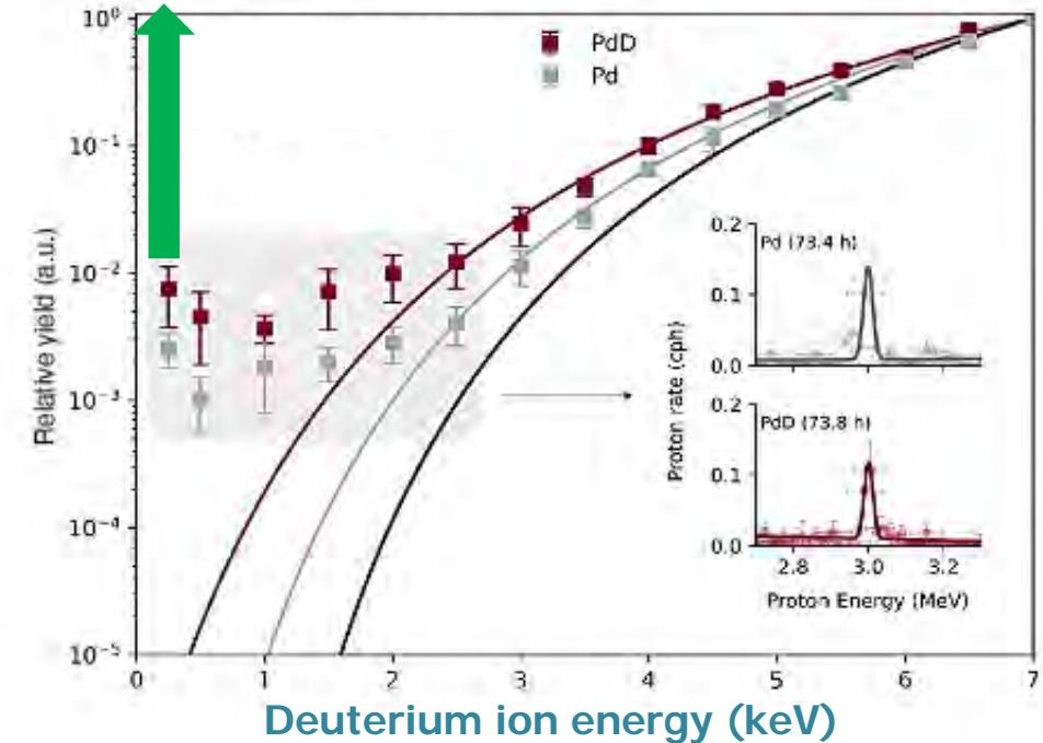
Deuterium-deuterium fusion yield as a function of ion beam trigger energy in palladium. The fusion yield near room temperature corresponds to a cross section of  $\sim 2 \times 10^{-13}$  barn.
