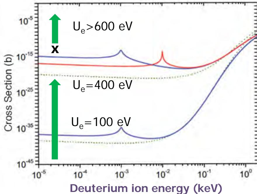
Non-resonant (dotted) and resonant (solid) cross sections for  $U_e = 400$  eV (upper) and  $U_e = 100$  eV (lower). Blue: resonance energy of 1 eV, red: 10 eV. Prediction of  $\geq 1$  Watt/gram for  $10^{-13}$  barn in "properly loaded metal".
