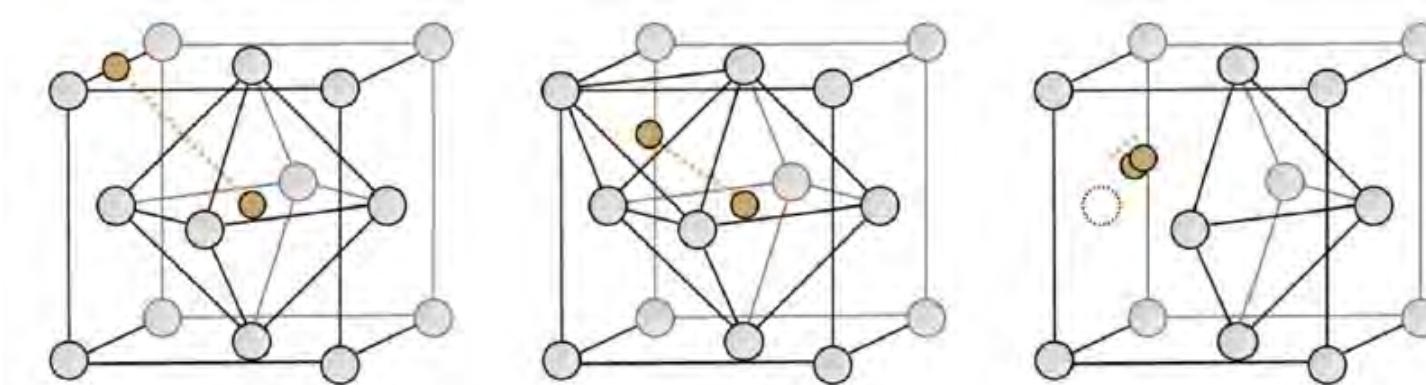
Configurations of deuterium atoms in the palladium lattice. Right: a deuterium pair trapped in a vacancy. We can tap into hydrogen storage science.
