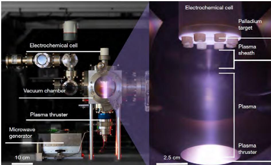
A membrane reactor integrated with a vacuum chamber. Demonstration fusion rate increases due to electro-chemical fuel loading in a beam driven fusion experiment (15 keV).
