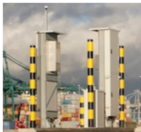
Arktis Radiation Detectors deployed operationally at the Port of Antwerp, Belgium
