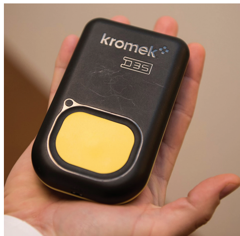
The SIGMA program delivered compact, inexpensive, and networked radiation detectors like this one that are now becoming part of the security infrastructure.
