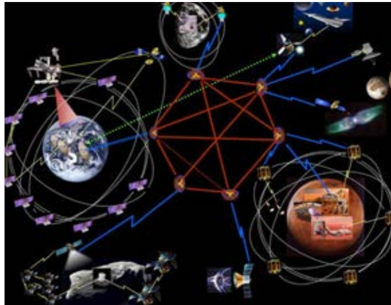
The Disruption Tolerant Network protocols will enable the Solar System Internet, allowing data to be stored in nodes until transmission is successful.
