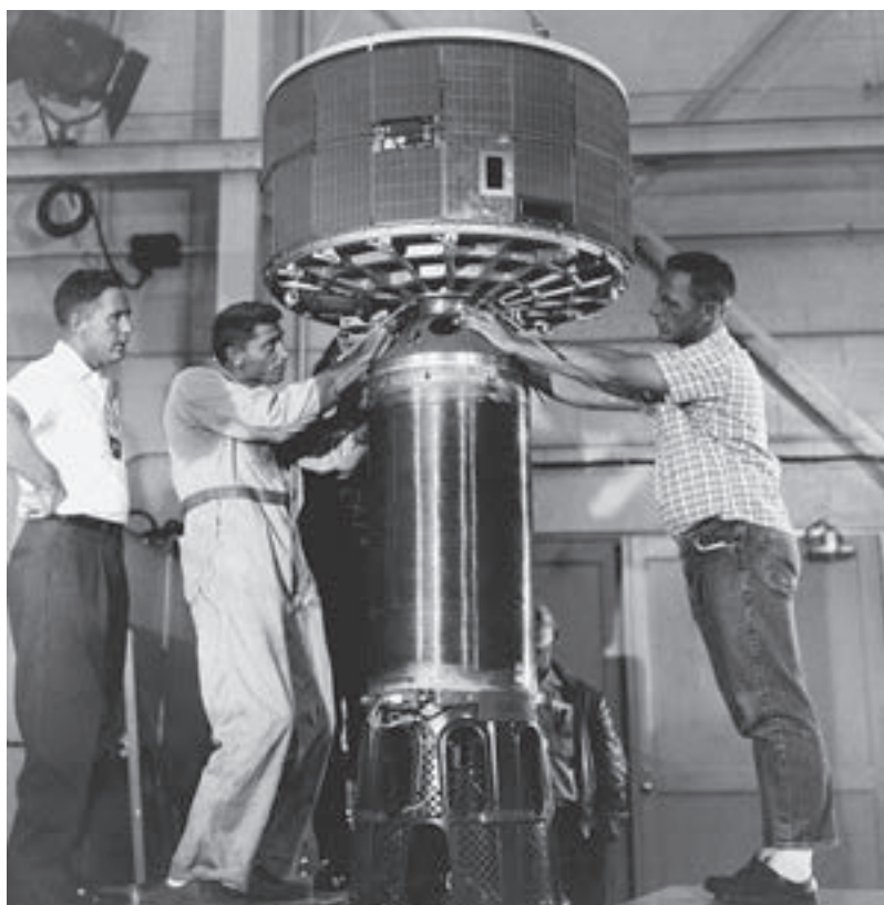
LEFT: Scientists prepare the first navigation satellite, Transit, for launch. Piggybacking on the spiral-adorned Transit was the Naval Research Laboratory's Solrad 1, a satellite with the dual purpose of measuring solar radiation and listening in on Soviet radar emissions. ABOVE: In the days before clean rooms, technicians work on the nation's first weather satellite, the Television Infrared Observation Satellite (TIROS).
