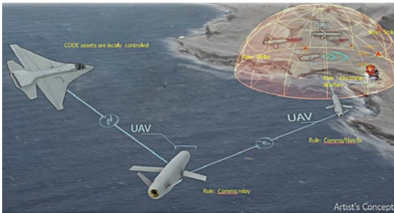
An artist's conception of manned and unmanned aircraft working cooperatively as envisioned in the Collaborative Operations in Denied Environment (CODE) program. CODE intends to focus on developing and demonstrating improvements in collaborative autonomy: the capability for groups of UAS to work together under a single human commander's supervision.
