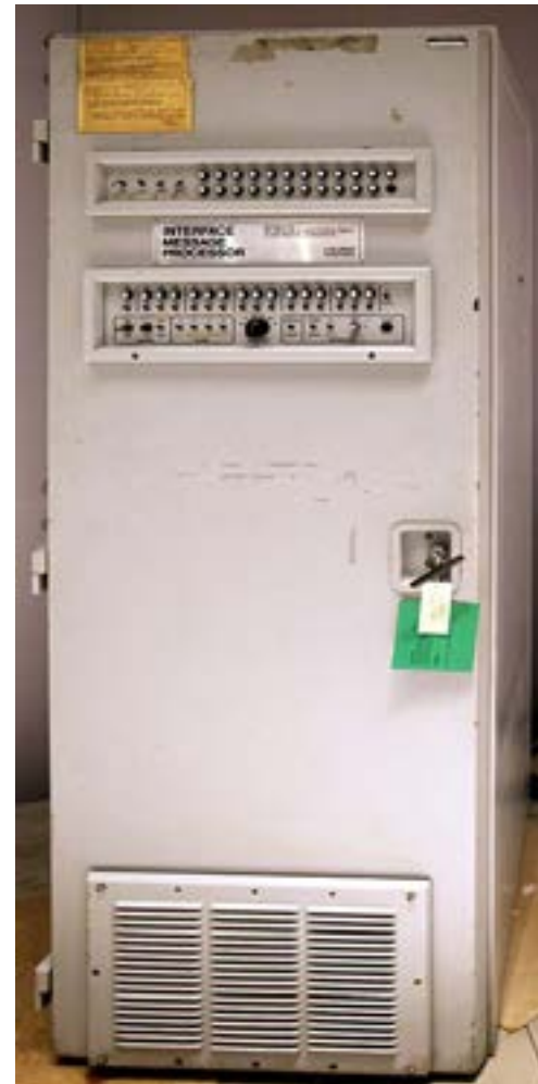
One of the many essential steps in the creation of what would become known as the internet occurred in 1968 when ARPA contracted BBN Technologies to build the first routers, known as Interface Message Processors or IMPs, which enabled ARPANET to become operational the following year. (Photo courtesy of Steve Jurvetson under a CC BY 2.0 license)
