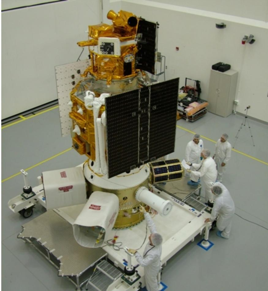
Fig. 1. Figure 1 is a picture of the NextSat vehicle atop the ASTRO vehicle in preparation for launch. The stack launched mated on an Atlas V launch vehicle on March 9, 2007.
